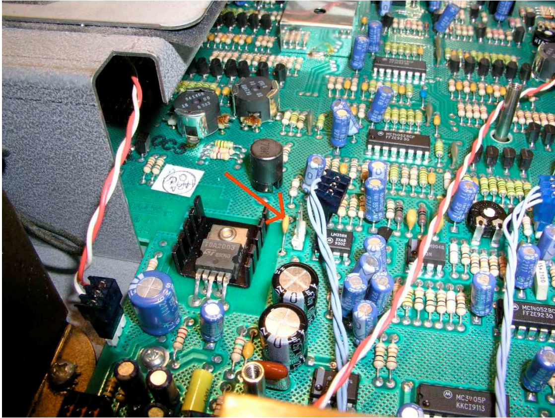
Picture 6 C137, plug P106 removed
