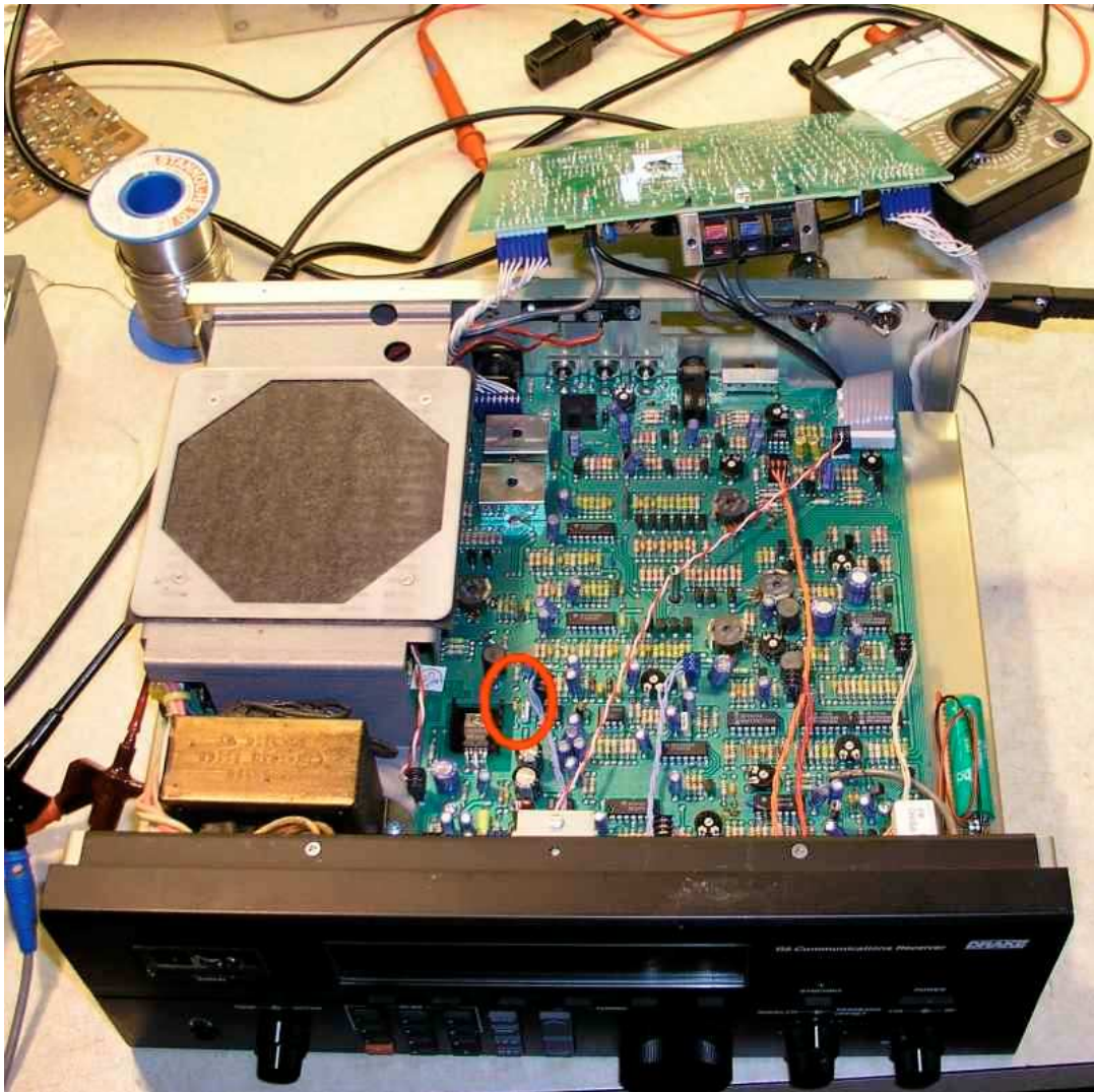
Picture 5 Location of C137 (front end board removed)
