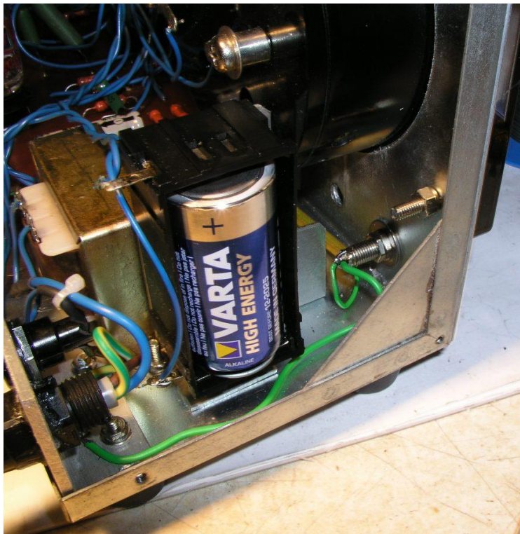
Picture 6: New case connector (right with green wire)
