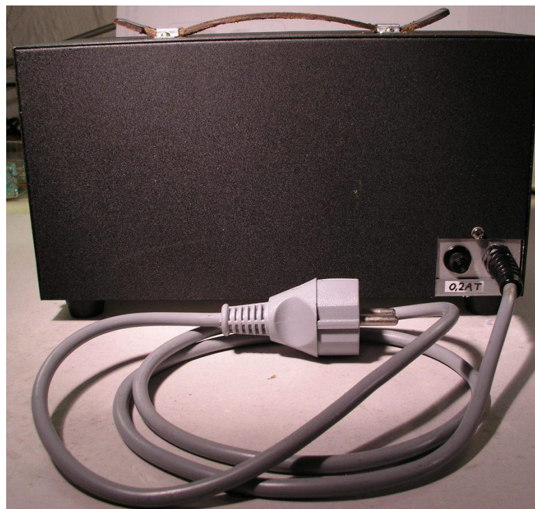
Picture 10: New line cord; 3-wire with protective ground
